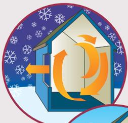
**U-Value:** A measure of the rate of non-solar heat loss or gain through a material or assembly. Tests are usually performed under conditions which simulate 0° outside and 70° inside with a 15 MPH wind. The lower a U-Value, the greater a window's resistance to heat flow, and thus the better its insulating value.
